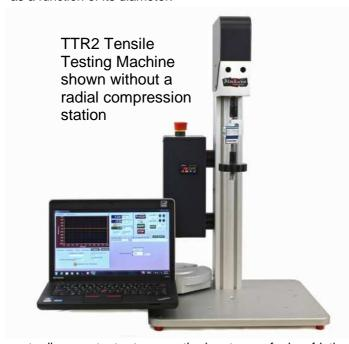
Radial Force is defined as total force transmitted in the radial direction across the (roughly) cylindrical outer surface of the device. It is equal to the average pressure on the surface times the surface area of the cylinder, and is also equal to the sum of the individual forces perpendicular to each of the die faces.
