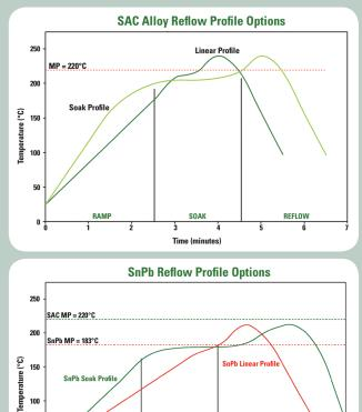
Peak reflow temperature should be <350°C in an air or nitrogen atmosphere, with a linear ramp up to
